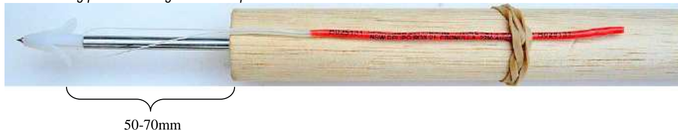
A finished tag pole with a tag secured in place with a rubber band
